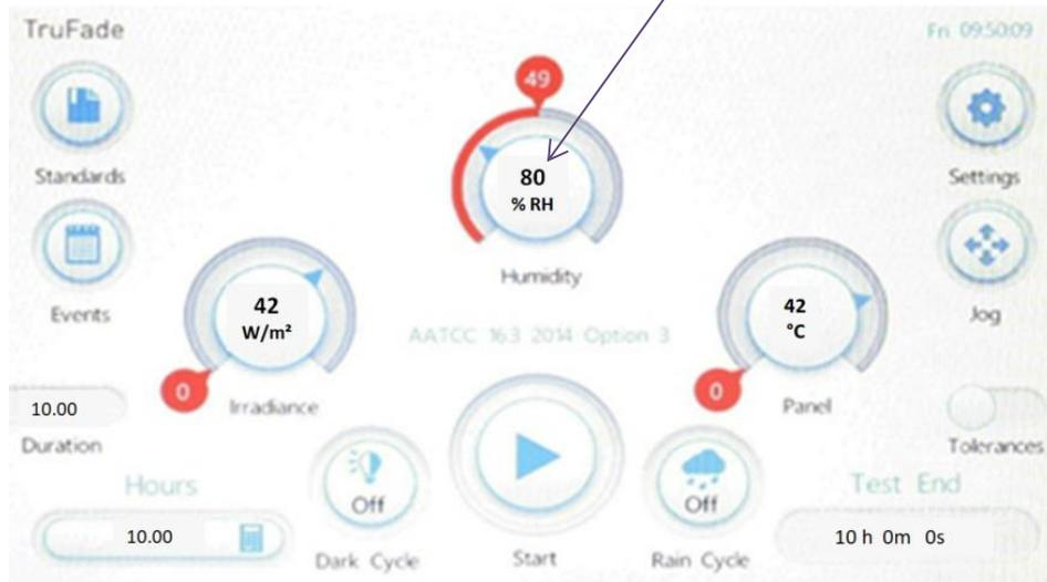
If the humidity test control fabric (red azoic) has faded less than the blue wool then the effective humidity is too low & so needs increasing on the dial (illustration only).
