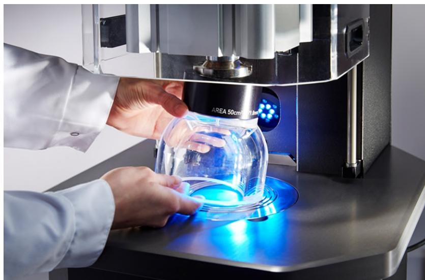
Remove the test dome from the end of the clamp piston by carefully pulling downwards; the dome is held secure by magnetic force.
