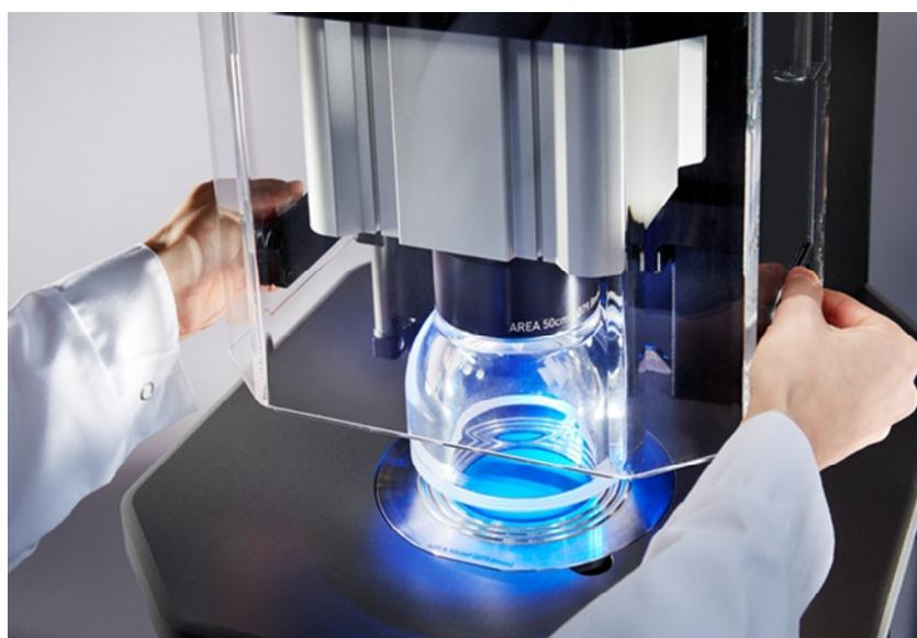
Standing in front of the instrument, using both side handles, slide the safety guard upwards until it locks into place.
