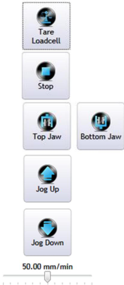
Tares the loadcell reading, resets the force to zero.
