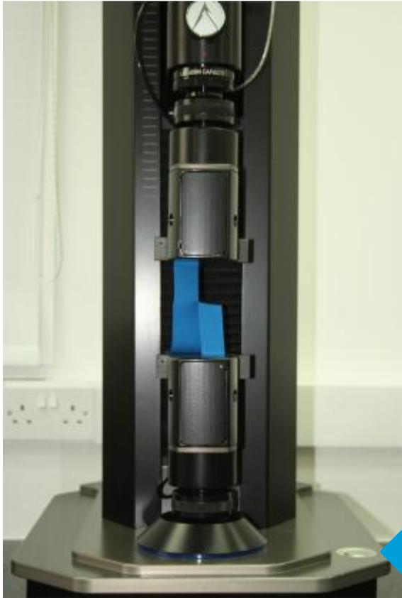
Position the specimen and close the **Top Jaw** and then the **Bottom Jaw**.
