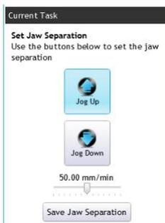
Adjust the jaw separation distance so that the hank can be placed on the Skein Spools by using **Jog Up** or **Jog Down** buttons.
