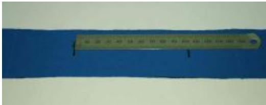
If Recovered Elongation is required, measure the gauge marks at the specified periods. In this example we used 60s (1 minute).
