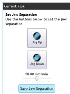
When the jaw separation is correct, click **Save Jaw Separation**.
