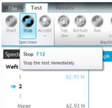
Observe the specimen as the yarns break. When the tear reaches the mark (25mm from the end of the specimen), click **Stop** or press the F12 function key.
