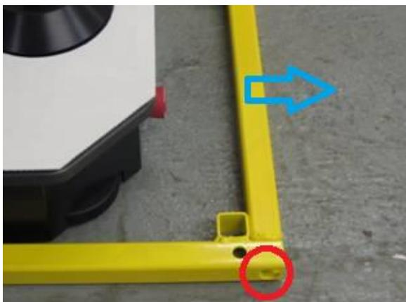
Once raised into the upright position, the bottom Yellow Transport Frame can be removed from the base by unbolting the front cross member (unscrew the bolts on the left and right as indicated by the red circle).
