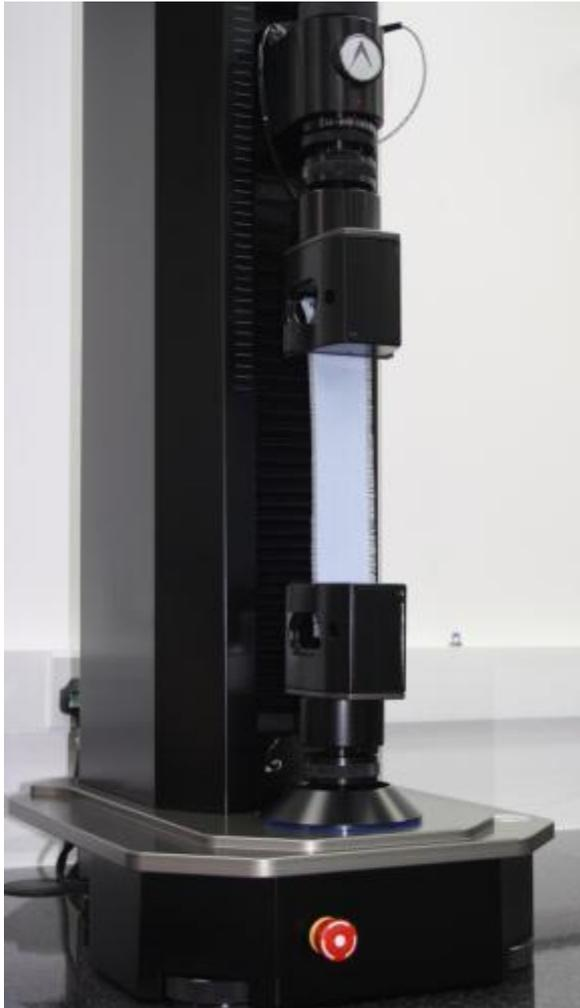
Specimen in the jaws ready for testing
