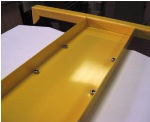
The top Yellow Transport Frame can now be removed from the instrument.
