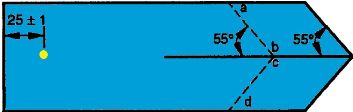
The lines a-b and c-d are lined up parallel to the edge of the jaw faces.
