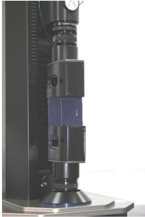
Specimen in the jaws ready for testing
