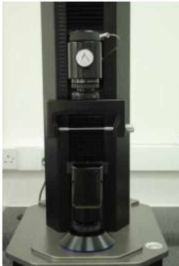
Then use the Jog Up and Jog Down buttons to move the top and bottom Jaw connections to a suitable position for fitting the new Jaws.
