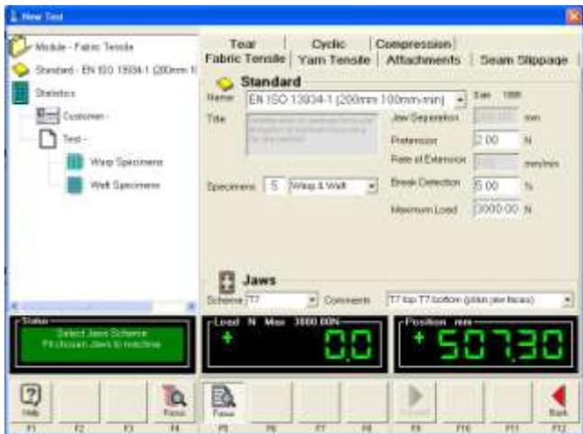
From the drop down list select the required **Standard** (test method).
