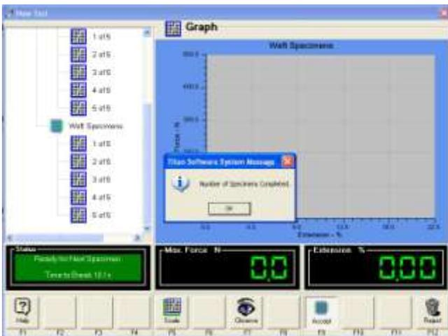
When all the required specimens have been tested the message "Number of Specimens Completed". Press OK to continue.
