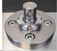
b) Sit the grip onto the top of the bottom adaptor, pushing the pin through the grip and then tightening the C spanner.
