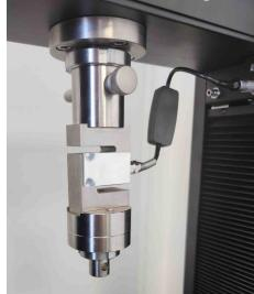
b) Using the adaptor 705-725, push this onto the bottom of the load cell and insert the pin through the hole and tighten the locking nut using the C spanner.
