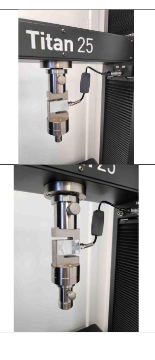
c) Place the grip onto the bottom of the adaptor, aligning the square ensuring it is in the correct orientation.
