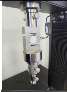
d) Place the grip onto the top of the adaptor, aligning the square ensuring it is in the correct orientation.
