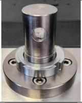
b) Connect the adaptor (705-725) to the bottom of the instrument by inserting it onto the post, push the pin through the adaptors and tighten the locking nut using a C spanner.
