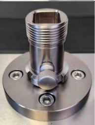
3. Place the grip onto the top of the adaptor, aligning the square ensuring it is in the correct orientation.
