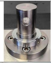
2. Connecting the 1710 Titan 5 tooling to the instrument requires a 31.8mm to 15.9mm conversion adaptor (stock code 705-723). Put the adaptor onto the bottom connector, push the pin through the adaptor and connector until it is through to the other side. Screw the locking nut up into place and tighten using the C spanner.
