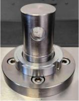
Connect the adaptor (705-725) to the bottom of the instrument by inserting it onto the post, push the pin through the adaptors and tighten the locking nut using a C spanner.
