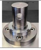
2. Connecting the 1710 Titan 5 tooling to the instrument requires a 31.8mm to 20mm conversion adaptor (stock code 705-724). Put the adaptor onto the bottom connector, push the pin through the adaptor and connector until it is through to the other side.
