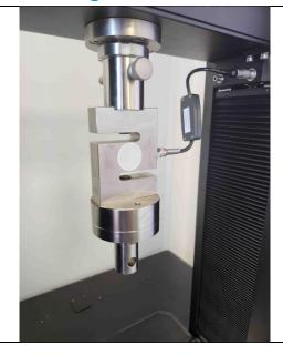
b) Using the adaptor 705-725, push this onto the bottom of the load cell and insert the pin through the hole and tighten the locking nut using the C spanner.
