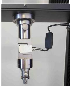
c) Push the grip onto the top of the adaptor in the same way, insert the pin through the grip and then tightening the locking nut with the C spanner.
