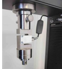
c) Push the grip onto the top of the adaptor in the same way, pushing the pin through the grip and then tightening the C spanner.
