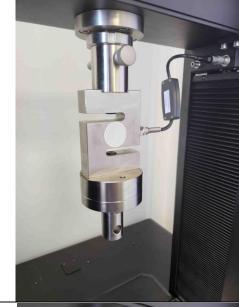
b) Connect a 31.8mm to 20mm adaptor to the bottom of the load cell and slide the pin through the adaptor, load cell and back through to the other side of the adaptor.
