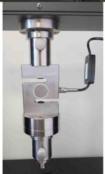
c) Push the grip onto the top of the adaptor in the same way, pushing the pin through the grip and then tightening the C spanner.
