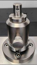
b) Sit the grip onto the top of the bottom adaptor, pushing the pin through the grip and then tightening the C spanner.
