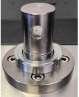
b) Sit the grip onto the top of the bottom adaptor, pushing the pin through the grip and then tightening the C spanner.
