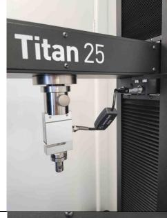
c) Push the grip onto the top of the adaptor in the same way, pushing the pin through the grip and then tightening the C spanner.
