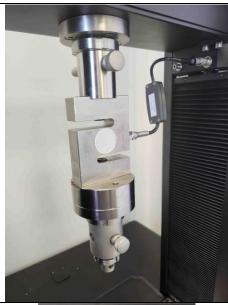
c) Push the grip onto the top of the adaptor in the same way, pushing the pin through the grip and then tightening the C spanner.
