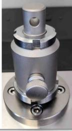
b) Sit the grip onto the top of the bottom adaptor, pushing the pin through the grip and then tightening the C spanner.
