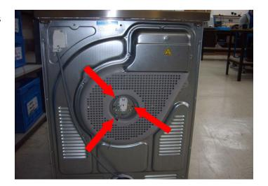
Remove the 7 screws holding the metal duct at the rear of the dryer.
