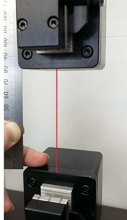
Move to top T38 grip to within 50 to 100 mm of the bottom grip.
