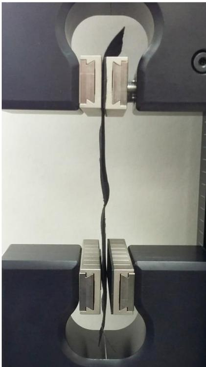
To permit the specimen to be slack mounted it must not be in contact with the body of the Grip. It should be suspended and hanging under its own weight only.
