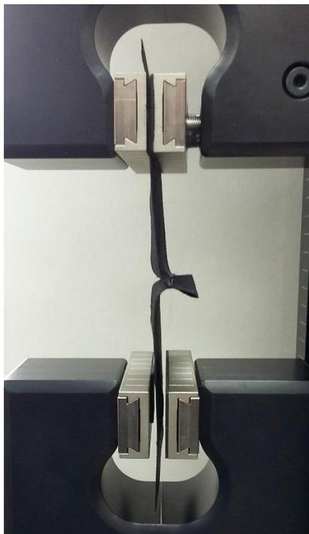
To permit the specimen to be slack mounted it must not be in contact with the body of the Grip. It should be suspended and hanging under its own weight only.
