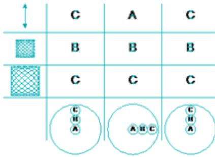
Assemble the Martindale Abrasion Tester so that all three (3) of the Drive Pegs are in position C indicated in the diagram to the left.
