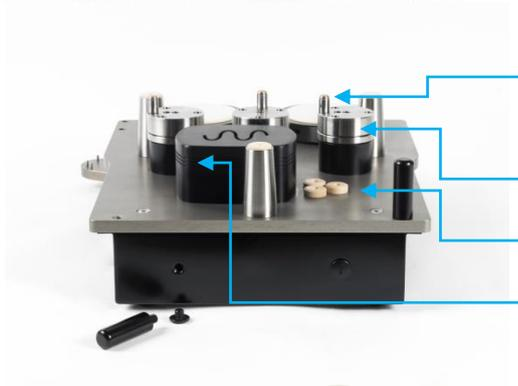
Drive Pegs (position can be changed to allow different types of motion)
