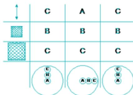
The instrument is supplied with the Drive Pegs in position C ready for abrasion testing. To change the motion, remove the Top Plate and set the Drive Pegs as required: Straight Line, 24mm Lissajous or 60.5mm Lissajous.
