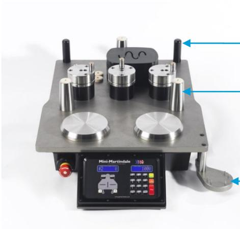
Unscrew the two (2) Support Bars and screw into the rear of the instruments. In this way they act as spacers giving adequate clearance at the rear of the instrument.
