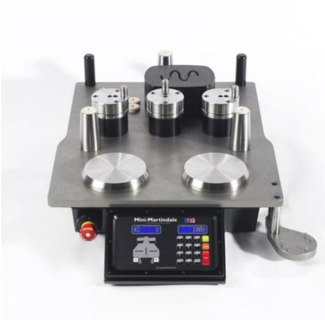
Ensure the Abrading Tables are free from adhesive residues.
