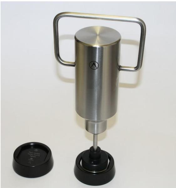
If using the 5.5 kg Weight, place the Weight on to the Spindle and tighten the Sample Holder
