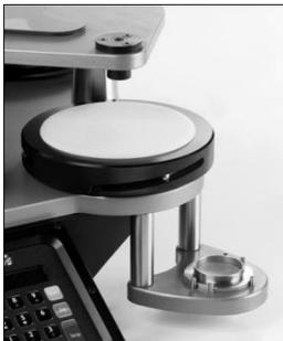
Place the 38mm diameter piece of Polyetherurethane (PU) Foam centrally into the Sample Holder Nut on top of the specimen.
