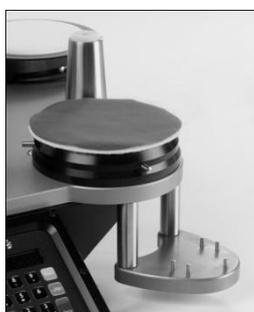
The pilling test can be carried out in two (2) ways: with Abrasive Cloth or with another specimen from the test sample. In this case we are showing a pilling test for apparel fabric.
