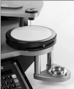
Place the 38mm diameter specimen, face down, centrally into the Sample Holder Nut.
