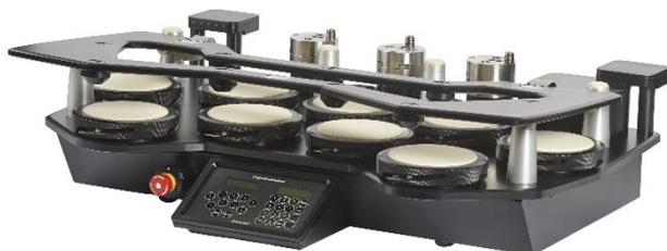
The smaller back part can be lifted away to allow access to the Drive Pins to change the motion of the Martindale.
