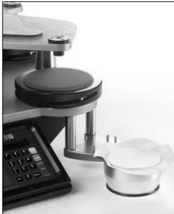
Place the Pilling Sample Holder centrally down on the Specimen and Felt.
