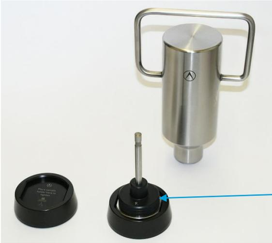
Assemble the Sample Holder in the Block Spanner in the usual way but do not tighten if using the 5.5 kg Weight
