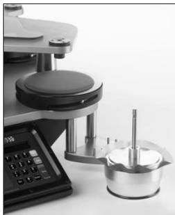
Gently press the Sample Holder against the Specimen Mounting Mandrel (use your thumbs to do this) while at the same time rolling up the black rubber Retaining Ring until it grips the Specimen on to the Pilling Sample Holder.
