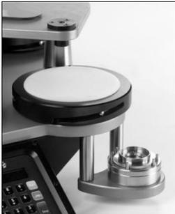
Place the 38mm diameter specimen, face down, centrally into the modified Sample Holder Nut.
