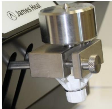
The rubbing finger can be removed by turning the “clamp screw” anti-clockwise until the clamping pressure is released. Replace the rubbing finger. Apply clamping pressure to secure the finger by turning the clamp screw clockwise.
