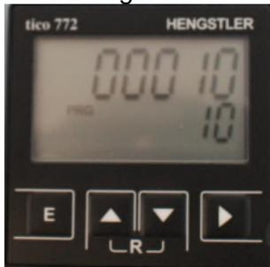
Use the right-arrow key in the programming mode to change a setting position. The selected position will start to flash.
