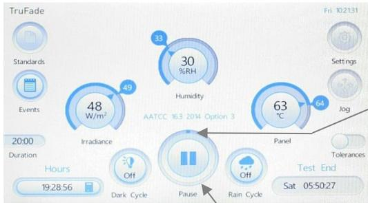
Notice the progress of the test (elapsed time) is also indicated on the Pause Dial.
