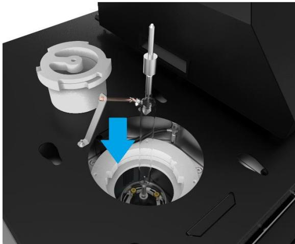
The Operator must place the xenon lamp with the larger diameter connector in first (at the bottom) and ensure that the lamp electrodes fits correctly, and tightly, onto the top end connection of the lamp.
