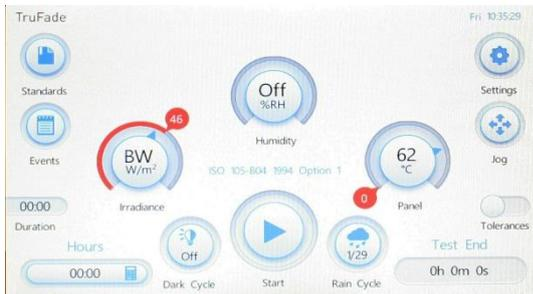
To change the parameter setting values for Relative Humidity, Temperature and Irradiance, tap the required Dial.
