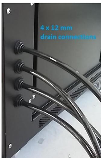
There are four (4) connections  $\varnothing$ 12mm for water drains.
