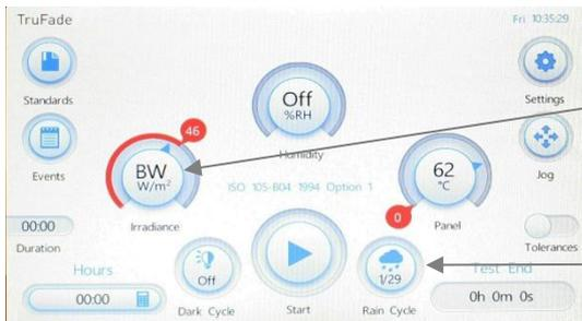
To changes from Controlled Irradiance mode to Blue Wool mode (nominal power), press and hold the Irradiance Dial
