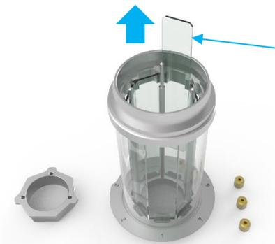
Carefully lift out the Optical Filter(s) and place on the bench.
