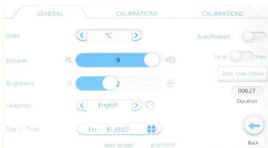
View and reset (zero) the Xenon Lamp and Filter timers.
