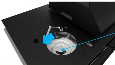
Rotate the PTFE Electrode Holder anti-clockwise by ¼ turn
