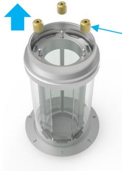
Unscrew the three (3) knurled brass nuts by hand, and place on the bench
