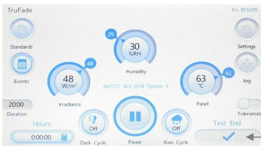
When the test Duration time has elapsed, the Test End will display "✓"
