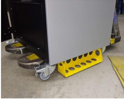
Use a pallet truck to lift the TruFade down the ramp.
