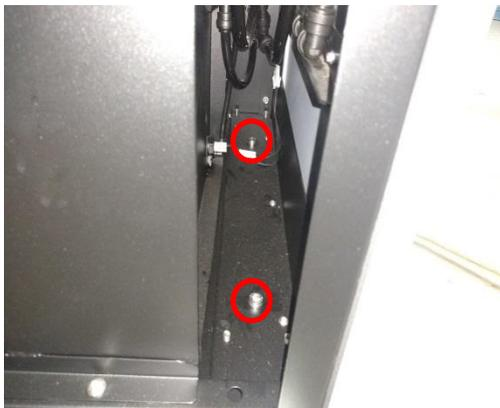
With the machine unwrapped, the transit frames will need to be removed.
