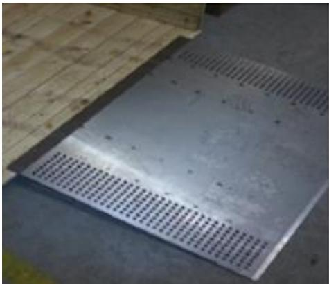
Position the ramp on the front of the box so that the instrument can be reached with a pallet truck.
