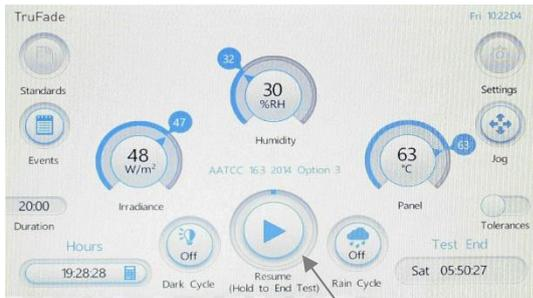
The test stops and the Xenon Lamp is switched off.
