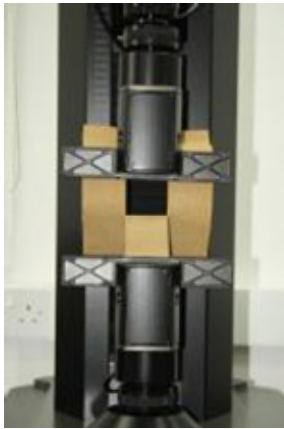
Tongue tear (or double-rip) tear specimen ISO 13937-4
