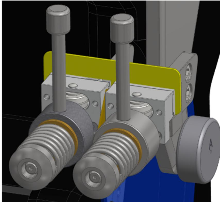
The optional E pendulum kit contains serrated jaw faces which provide additional specimen gripping at high tearing forces.
