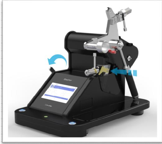
Raise the blade by using the blade handle on the left hand side of the instrument. Remove the blade by loosening the screws, and replace with a new blade.
