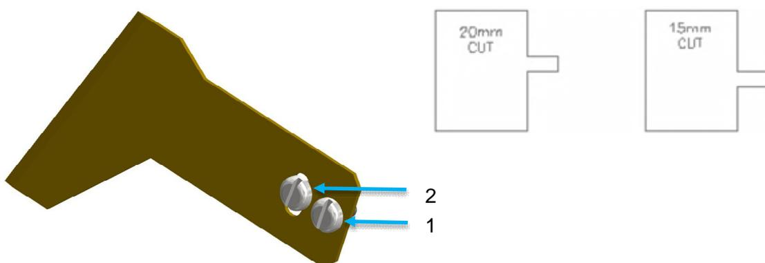
Loosen both screws by turning counter clockwise, sufficient to allow the blade to pivot.
