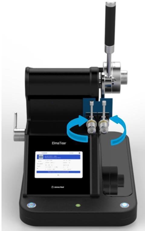
Place a test specimen centrally in the jaws so that the specimen is set carefully against the bottom of the jaws.
