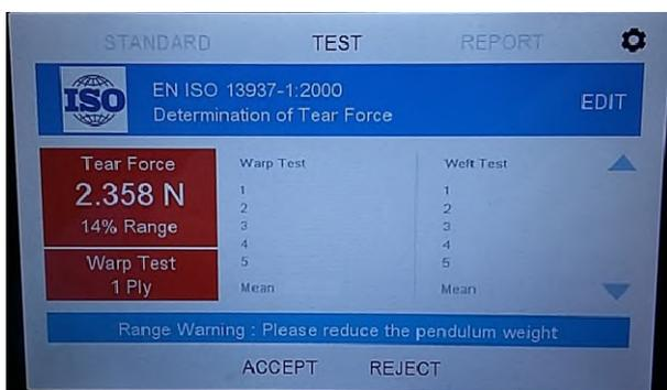
ElmaTear will also provide advice on if to reduce or increase the pendulum weight. The operator can then choose to Accept or Reject the test result.
