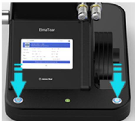
Please press both buttons at the same time to release the pendulum.
